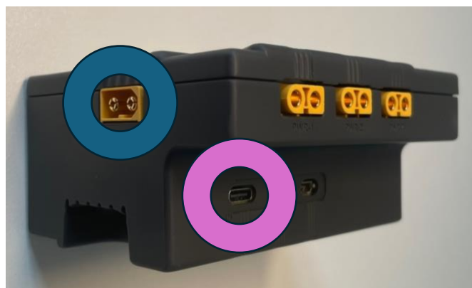
Figure 2. Location of input power. Provide 12v input via the male XT60 connector circled in blue, or 5v through the USB-C port circled in purple.
