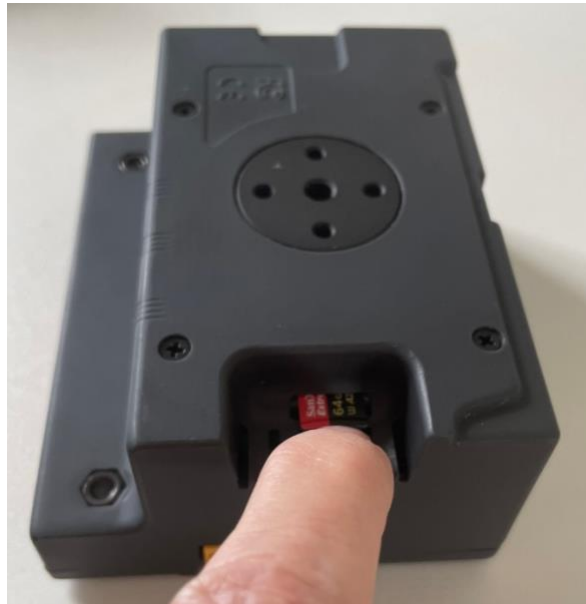
Figure 1. Location of the SD card slot. The electrical connectors should face downwards and be inserted into the slot. The lip on the SD card will allow you to remove the card if necessary.
